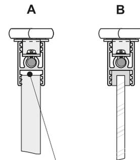
Expansion gap taken into account when calculating the height of chipboard
